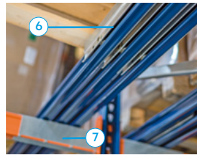
Rails et supports de rail
